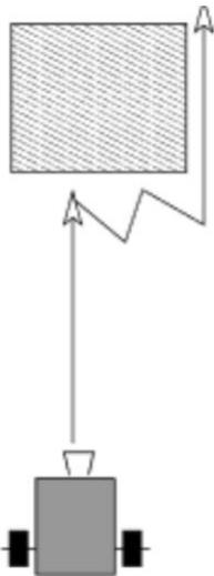
The robot should move up until it is close to the obstacle and wiggle it's way around it.
