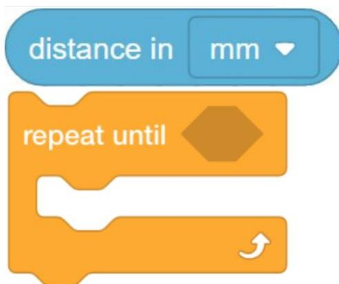
If the robot is too close into an object, have the robot go around the object. Have a threshold to see if the distance is below a certain amount that is considered close. Do not bump into an object.
